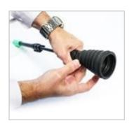
Unscrew and remove the rubber housing from the end of the sample probe.
