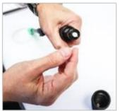
Once the rubber housing has been removed, remove and discard the cellulose filter from the holder found at the end of the wand
