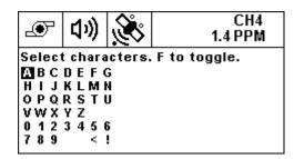
• Rotate the Selector dial to select a character of the Pol name and press the Selector to enter that character. The display will update and show you any potential matches. In this case, the starting letter 'S' matches to 3 points in the instrument's data set.
