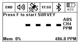
• Field calibration is now complete and the calculated exceedance value is displayed in the lower right corner
