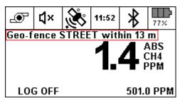
The instrument does not automatically record any data against these fences; they are used primarily for ease of location for operators.
