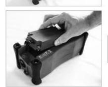
Replace with fully charged battery and tighten screws
