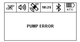
The instrument detects when the pump flow is restricted or blocked. The pump stops, the LEDs light up, the icon of the pump shows a cross and you will see the message "PUMP ERROR" is displayed on the screen.
